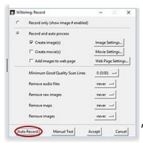
Go to File > Record and click on Auto Record, fig.26. The recording, decoding and imaging will start when the satellite appears on your horizon, and stop when it is out of sight according to the times stated in the satellite Satellite Pass List. After activating Auto Record, also in the bottom line of the "Wxtolmg" screen appears the message with the start and end time with the date of the next satellite pass recording, fig.26.
