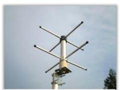
Figure 2, Turnstile antenna.
