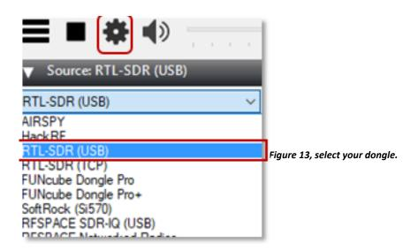
Important! don't forget to also adjust the RF Gain settings by clicking the Configure Source button. , fig.13. By default, the RF-Gain is set to zero.
