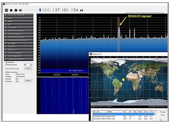
.Figure 29, SDRSharp in receive mode.
