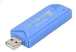
Figure 4, RTL-SDR dongle
