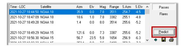
According to the timetable, fig.63, 'Orbitron' will automatically start up 'SDRSharp' at 5:41 PM and 7 seconds at the previously set frequency of the NOAA15.
